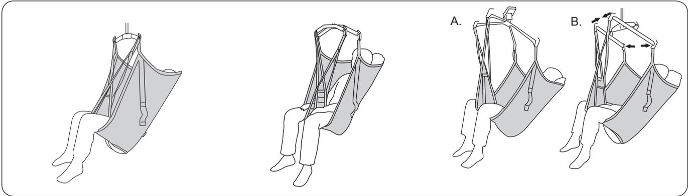
Liko Original HighBack Sling in **two-point suspension** provides for a slightly reclined sitting posture with excellent head support and approx. 90 degrees angle in the hip joint.
