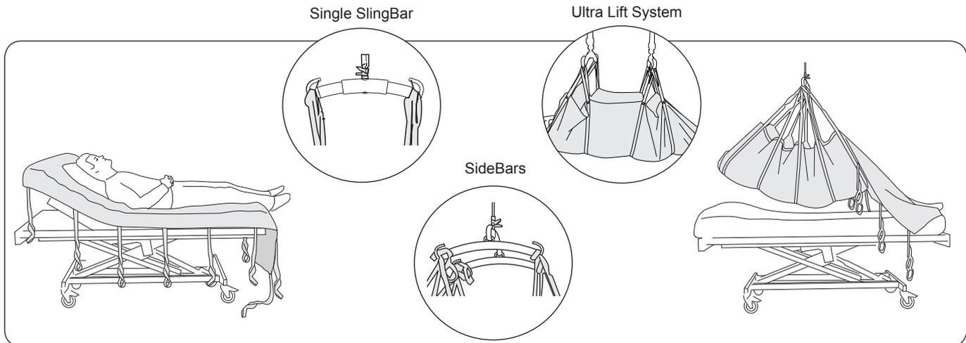
Hook the loop straps to the sling bar hooks on the respective sides (see the small illustrations). The lift straps are different colours to enable correct matching of lift straps pair-wise. Use the lift straps that lift the head and all of the lift straps that lift the body, as far down as the knees (normally 4-5 pairs of straps).
