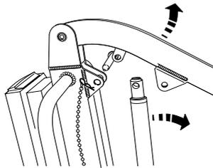
5. Remove the quick release pin at the top of the actuator, this will release both the boom and the actuator. Hydraulic version - The hydraulic unit is completely detached when the Stowaway is folded. Remove the quick release pin to release the boom and use the pin to reconnect the top of the hydraulic unit to the boom. Connect the lower mounting of the hydraulic unit to the mast with the second quick release pin stored through the mast bracket.
