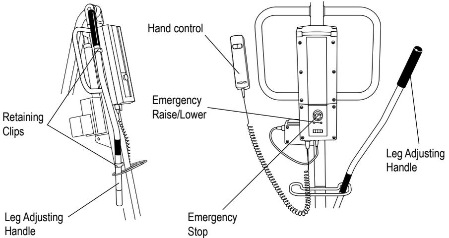
7. Remove leg adjusting handle from the storage clips on the mast and fit to the leg adjusting lever through the gate on the mast. Fit the battery pack to the mounting point on the mast and connect the power/charging plug to the battery pack.
