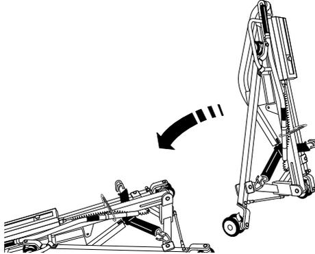
2. Place the folded Stowaway flat on the floor, resting on the rear castors and the folded boom. Engage the brakes on the rear castors.
