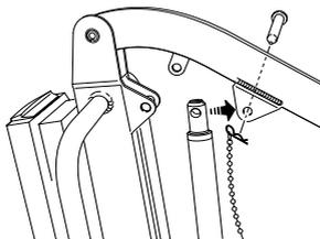
6. Lift the boom and spreader bar and swing the actuator over to engage with the mounting bracket on the underside of the boom. Secure the actuator to the boom mounting bracket with the quick release pin.
