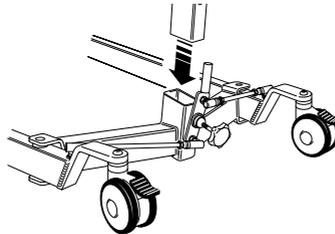
**SAFETY NOTE:** Avoid trapping fingers. Keep fingers away from the end of the mast when inserting into the socket.
