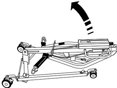
3. Stand facing the front castors and swing the leg retaining latches clear of the square handle on the mast. Move the legs sideways and downwards to place the front castors on the floor.
